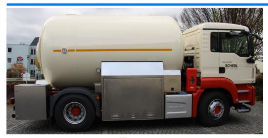
Fixed structure for 4x2 (4x4) bobtails with a total weight of 18 tons. The advantage of a fixed structure is a low-lying stainless steel cabinet on a side of the vehicle. It is a very compact solution with compressor.
